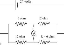
Q.19> In the circuit diagram, what is the reading of the voltmeter?
