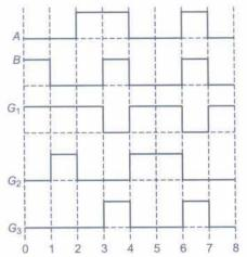
(b) The inputs, A and B, shown here, are used as the inputs for three different gates,  $G_1$ ,  $G_2$  and  $G_3$ . One by one. The outputs, obtained in the three cases, have the forms shown. Identify the three gates and write their symbols.
