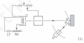
The accelerated electron beam strikes to nickel crystal and get scattered in different directions. The intensity of scattered electron beam can be obtained by detecter.
