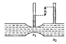
Two manometers are mounted on a horizontal pipe carrying water at the positions where the areas of cross-sections of the pipe are  $s_1$  and  $s_2$  as shown in the figure. If the difference in water column at these cross-sections is h, what is the volume of water flowing through the pipe per unit time?
