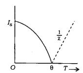
The variation of magnetization with temperature (T) of a magnetic material is shown in the figure. As the temperature increases, the magnetization drops down to zero at Curie temperature  $\theta$ . Above Curie temperature,  $1/\chi$  (where  $\chi$  is the susceptibility) increases linearly with temperature. What would be the nature of magnetic material?
