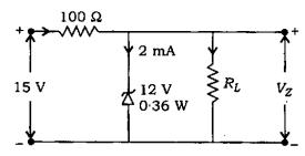
In the above circuit, what is the range over which the load resistance can be varied?
