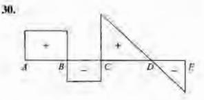
Consider the following statements with reference to a continuous beam supported at A, C and E for which shear force diagram is shown in the above figure.
