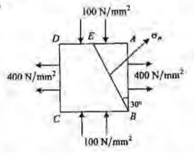
The principal stresses in N/mm<sup>2</sup> on a rectangular element are shown in the above figure. The intensity of normal stress  $\sigma_n$  on the oblique plane *BE* is
