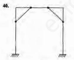
The degree of static indeterminacy for the rigid frame as shown above is
