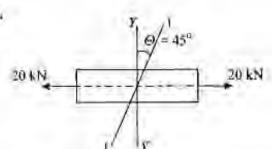
A mild steel har of square cross-section has a sectional area 200 mm<sup>2</sup>. It is subjected to an axial force of 20 kN as shown in the above figure. The intensity of the normal tensile stress is N/mm<sup>2</sup> on the oblique plane 1-1 at 45° with the *YY*-axis which is normal to the longitudinal axis will be
