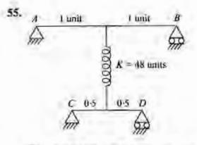
The equivalent spring constant for the set up shown in the above figure, where EI = unity throughout, is
