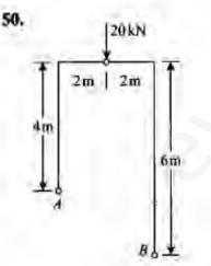
For the frame shown above, what is the horizontal thrust at A?
