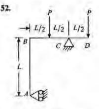
A frame ABCD is supported by a roller at A and is on a hinge at C as shown in the above figure. The reaction at the roller end A is given by
