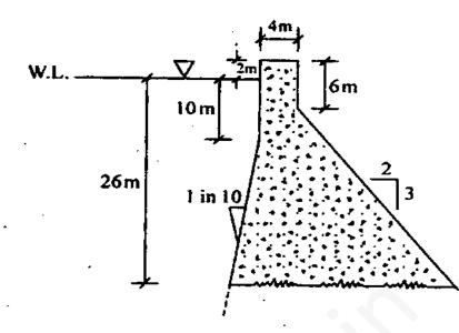
A part of a solid gravity dam (sp. gr. of mass concrete = 2.64) is shown in its cross-section. Take uplift factor as 0.7. Draw a tabular statement for analysis of forces at a horizontal section 26 m below water level. No ice, wind or seismic forces need to be considered. 20
