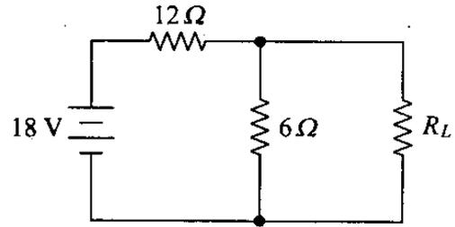
In the circuit shown above, the maximum power absorbed by the load resistance  $R_L$  is
