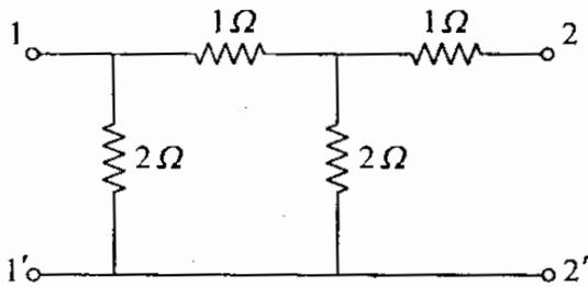
The Z-parameters of the 2-port network as shown above are
