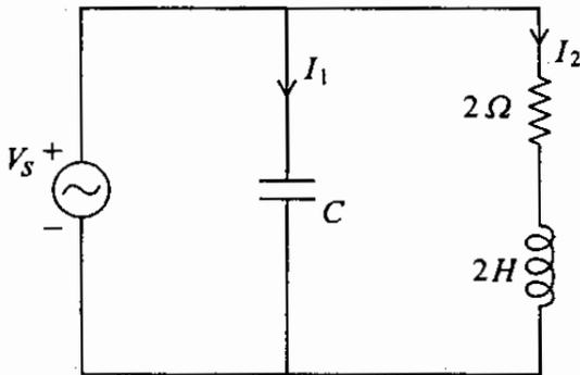
In the network shown above  $V_s = 4 \cos 2t$ . The value of  $C$  is so chosen that the circuit impedance is maximum. Then  $I_1$  leads  $I_2$  by
