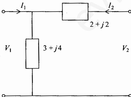
The Z-parameter matrix of the two-port network as shown above is
