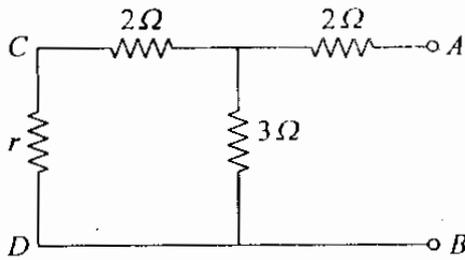
For the circuit shown above the value of  $r$  connected between  $C$  and  $D$  is such that the equivalent resistance of the circuit by looking into circuit through terminals  $A$  and  $B$  is  $r$  only. Then the value of  $r$  is
