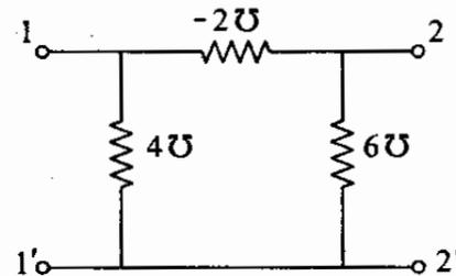
For the two port network as shown above, the parameters  $h_{11}$  and  $h_{21}$  are
