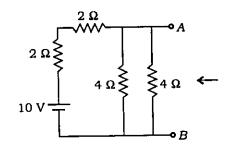
The output resistance of the circuit at port AB is
