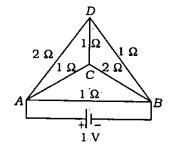
A triangular pyramid, built up of six wires whose resistances are shown in the figure, is fed from a 1 V battery at the terminals A and B. The current through the branch DB
