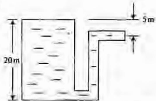
The velocity at the exit of the pipe as shown in the above figure will be
