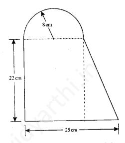
Compute second moment of area of the plane lamina shown in the above figure about an axis parallel to the base and passing through the centroid. 20
