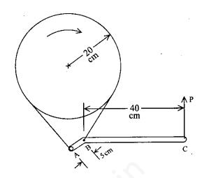
A band brake is used to stop a machine. The brake band is in contact with the brake drum through an angle of  $250^{\circ}$ . The coefficient of the friction is 0.3. Determine the force P required to develop the braking torque of magnitude 400 Nm. The arrangement is shown in the above figure. 12
