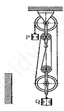
Figure shows a polyspast lifting a weight Q equalling 1000 N by another weight of P equalling 300 N. Neglecting friction and the masses of the pulleys and cables and the inclinations of cables, determine the distance moved by Q in 2 seconds from start.
