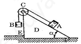
A body A weighing  $P_1$  descends down an inclined plane D which makes an angle  $\alpha$  with the horizontal and pulls a load B that weighs  $P_2$  by means of a weightless and inextensible string passing over a pulley C as shown in Figure. Determine the horizontal component of the pressure with which the inclined plane D acts on the floor rib E.
