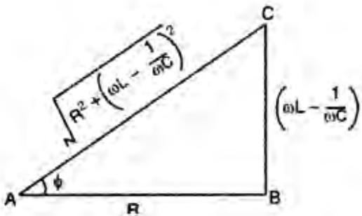
$$\sin \phi = \frac{\omega L - 1/\omega C}{\sqrt{R^2 + (\omega L - 1/\omega C)^2}}$$
