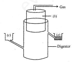
The diagram above is that of a typical biogas plant. Explain the sequence of events occurring in a biogas plant. Identify a, b and c.
