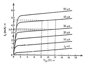
Output characteristics of an n-p-n transistor in CE configuration is shown in the figure. Determine:
