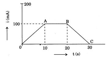
Calculate the value of E.C.E. of copper in terms of the mass, m, deposited.
