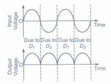
Its working based on the principle that junction diode offer very low resistance in forward bias and very high resistance in reverse bias.
