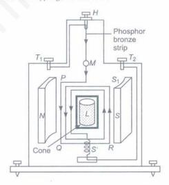
It is a device used to detect small current flowing in an electric circuit. With suitable modifications, a moving coil galvanometer can be used to measure current and potential difference.
