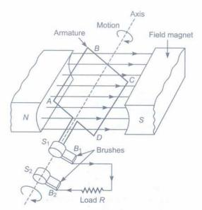
Principle AC generator works on the principle of electromagnetic induction. Whenever amount of magnetic flux linked with a coil changes an emf induced in the coil. It lasts so long as the change in magnetic flux through the coil continues.
