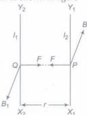
Let us find the force experienced per unit length by the current carrying conductor  $X_1Y_1$  due to the magnetic field produced by the current carrying conductor  $X_2Y_2$ .
