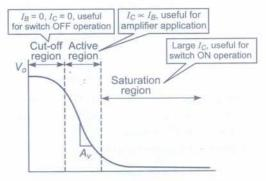
The active region of transfer characteristic curve operates as an amplifier.
