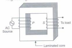
Working When an alternating current is passed through the primary, the magnetic flux through the iron core changes, which does two things. It produces emf in the primary and an induced emf is also set up in the secondary. If we assume that the resistance of primary is negligible, then the back emf will be equal to the voltage applied to the primary.
