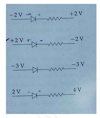
Sol. Toward biased connection, when positive terminal of the battery connected to the P-terminal source.
