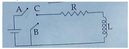
Sol. In (R-L) circuit, inductor would be charged first and then discharged later through resistance, R.
