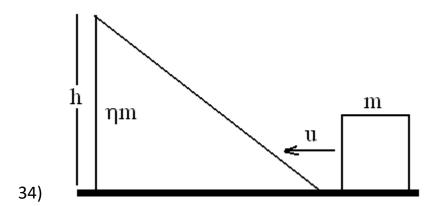
A block of mass m is pushed towards a movable wedge of mass  $\eta m$  and height h, with a velocity u. All surfaces are smooth. The minimum value of u for which the block will reach the top of the wedge is
