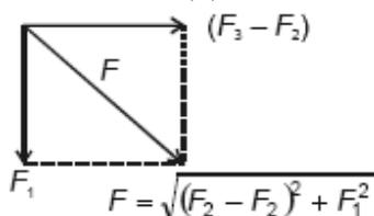
Since net force on current carrying loop in uniform magnetic field is zero therefore force on remaining segment will be equal and opposite to  $F$ .
