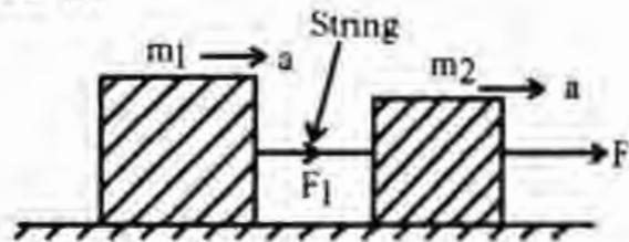
Refer to the figure. Let  $f$  be the frictional force on each block. Equations (i) and (ii) are modified to
