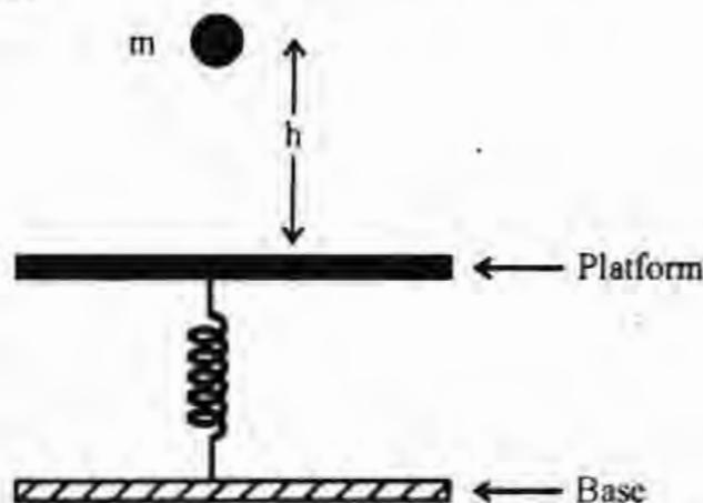
A body of mass  $m = 1\ \text{kg}$  is dropped from a height  $h = 40\ \text{cm}$  on a horizontal platform fixed to one end of an elastic spring, the other being fixed to a base,
