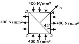
The square element in the figure is subjected to a biaxial stress of 400 N/mm<sup>2</sup> as shown. What is the intensity of normal stress  $p_n$  on the plane *BD*?
