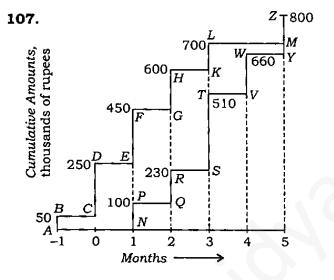
In a project of notional 4 months duration, the cumulative outgo and cumulative receipt of a contractor are shown. Outgo is through *ABCDEFGHKLM* and receipt is through *NPQRSTVWYZ*. Amounts are in thousands of rupees cumulative, as indicated. What is the working capital required?
