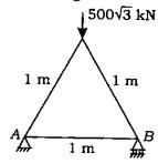
(Cross-sectional area of each member = 50 mm<sup>2</sup>, modulus of elasticity  $E = 2 \times 10^5$  N/mm<sup>2</sup>)
