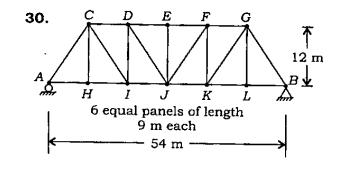
For the pin-jointed plane truss shown in the figure, which of the following diagrams represents the influence line for the bar force in the member *DI*, when a load travels on the bottom chord?
