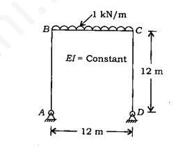
What is the bending moment at B for the symmetrical portal frame shown, which is subjected to a uniformly distributed load of 1 kN/m on the beam portion?
