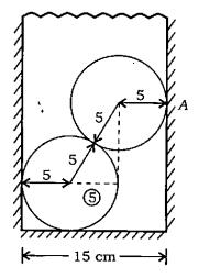
In the figure shown, consider the two identical spheres with radius 5 cm, weight 100 N each and the distance between the two walls as 15 cm. What is the reaction force at point A?
