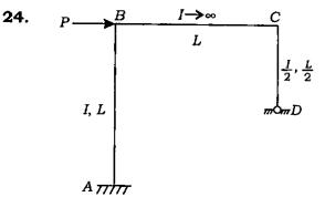
In the portal frame shown, find the ratio of moments  $M_{BA}$  and  $M_{CD}$  induced at the column heads due to sidesway
