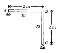
What is the force required for displacing support C horizontally through a distance  $\Delta$ ?
