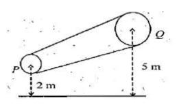
done per unit volume by the pressure and the gravity forces as the fluid flows from point P to Q (IIT JEE -1997 – 5 Marks)
