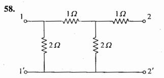
The Z-parameters of the 2-port network as shown above are
