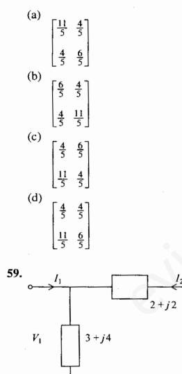
The Z-parameter matrix of the two-port network as shown above is
