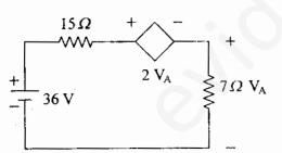
The power dissipated in the controlled source of the network shown above is
