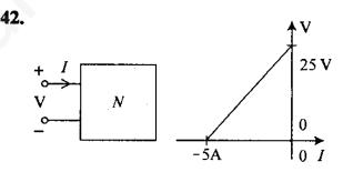
The voltage-current relationship feeding the network N is shown in the above figure. The Thevenin's equivalent of network N will have  $V_{Th}$  and  $R_{Th}$  as
