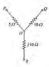
In the delta equivalent of the above star connected circuit,  $Z_{OR}$  is equal to
