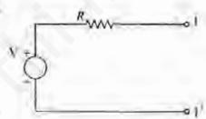
Thevenin equivalent circuit of a network N is shown above (at terminals  $1-1^1$ ).
