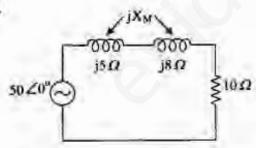
The power absorbed by the network excited by a  $50 \ge 0^{\circ}$  sinusoidal source is 168 W. The value of the mutual inductive reactance  $jX_M$  should be
