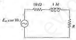
In the above circuit, the value of the load resistance R to absorb the maximum power is
