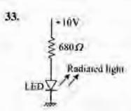
The Light Emitting Diode (LED), shown in the above figure has a voltage drop of 2 V. The current flowing through LED is
