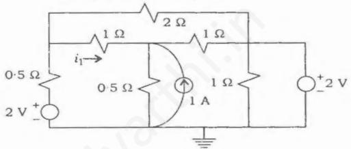
(ii) For the network shown below, write mesh equations in vector-matrix form for the loop currents  $i_1$  and  $i_2$ .
