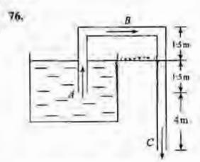
A tube is used (as shown in the above figure) as a siphon to discharge an oil of specific gravity 0.8 from a large open vessel into a drain at atmospheric pressure. The velocity of oil through the siphon will be
