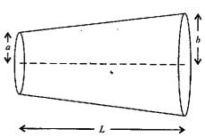
A resistor is in the shape of a truncated right circular cone as shown in the figure. The end radii are a and b, and the length is L. The specific resistance of the material is  $\rho$ . What is the resistance of the object? [Assume that the taper is small, so that the current density is uniform across any cross-section]
