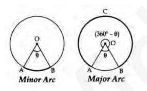
If the arc subtends angle ' $\theta$ ' at the centre, then the Length of minor arc =  $\frac{\theta}{360} \times 2\pi r = \frac{\theta}{180} \times \pi r$ Length of major arc =  $\left(\frac{360-\theta}{360}\right) \times 2\pi r$
