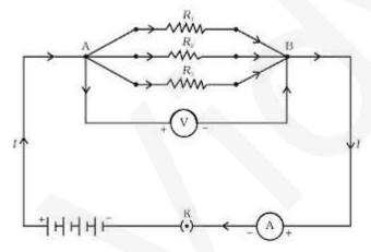
$\rightarrow$  Voltage across each resistor is same and equal to the applied voltage.
