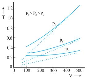
**Fig. 13.3** Experimental T-V curves (solid lines) for  $CO_2$  at three pressures compared with Charles' law (dotted lines). T is in units of 300 K and V in units of 0.13 litres.
