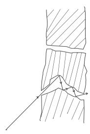
Fig. 13.5 Molecules going through a porous wall.
