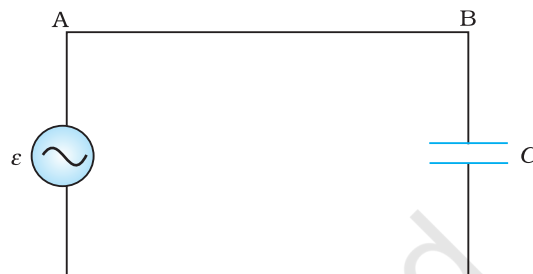
FIGURE 7.8 An ac source connected to a capacitor.
