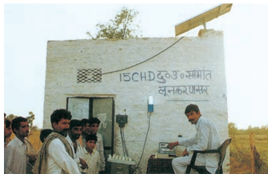
Fig. 5.10: Solar operated electronic milk testing equipment
