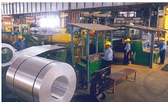
Fig. 6.3: Strip coating mill at smelter of NALCO
