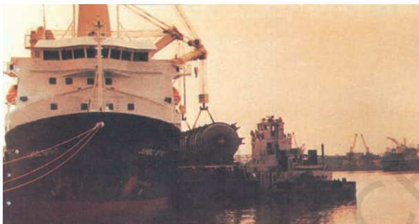
Fig. 7.8: Handling of oversize cargo at Tuticorin port
