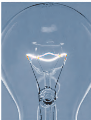
Fig. 10.12 Glowing filament of an electric bulb (incandescent)
