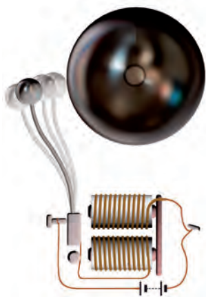
Fig. 10. 20 Circuit of an electric bell
