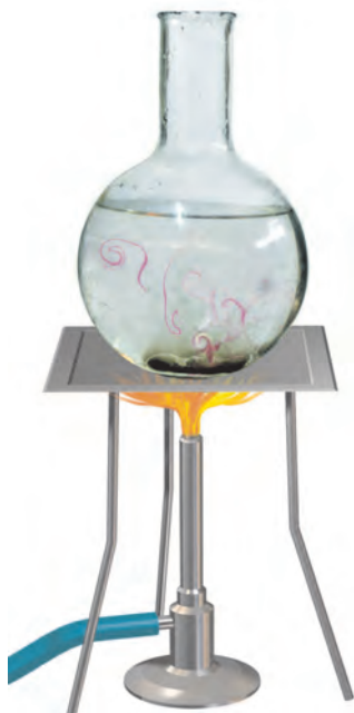
Fig. 3.9 Convection of heat in water
