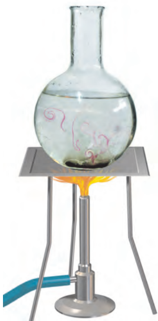
Fig. 4.9 Convection of heat in water
