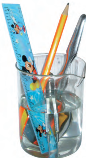
Fig. 4.8 Conduction of heat by different materials
