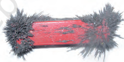
Fig. 10.7 Iron filings sticking to a bar magnet
