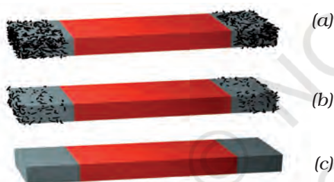
Fig. 10.6 Magnet with (a) many iron filings (b) few iron filings and (c) no iron filings sticking to it.
