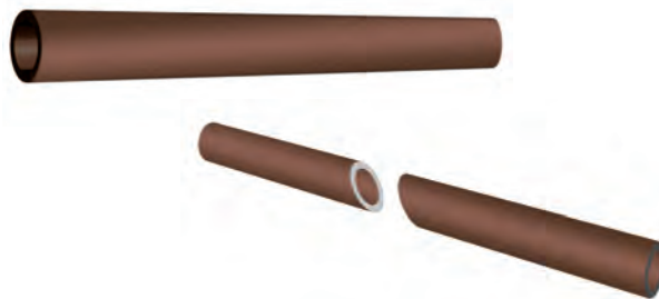
Fig. 2.3 Cutting pieces of materials to see if they have lustre
