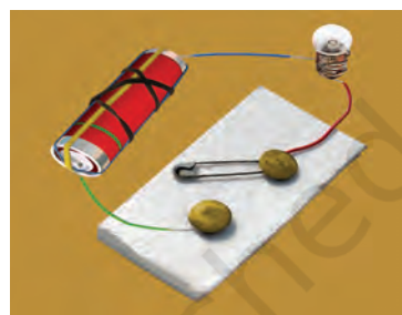
Fig. 9.9 An electric circuit with a switch
