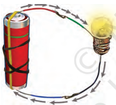
Fig.9.6 Direction of current in an electric circuit
