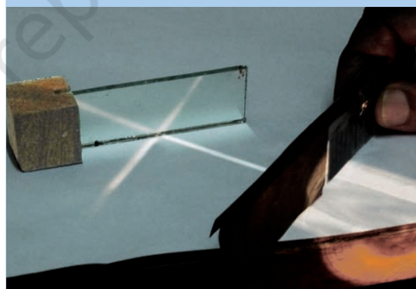
Fig. 13.1 : Arrangement for showing reflection
