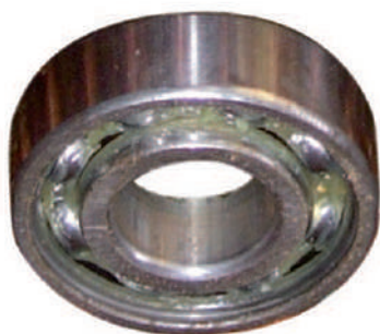
Fig. 9.16 : Ball bearings reduce friction
