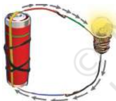
Fig.12.6 Direction of current in an electric circuit
