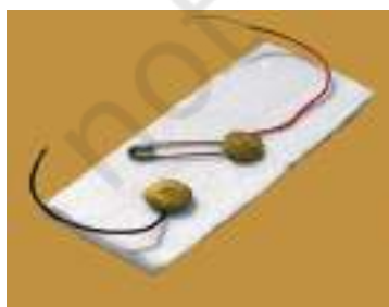
Fig. 12.8 A simple switch
