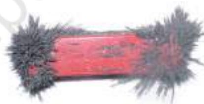
Fig. 13.7 Iron filings sticking to a bar magnet
