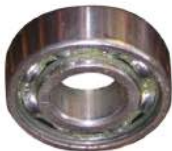
Fig. 12.16 : Ball bearings reduce friction
