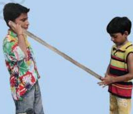
Fig. 13.12 : Sound travelling through a metre scale
