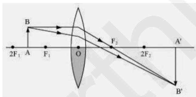
$$\begin{aligned} \frac{1}{v} - \frac{1}{u} &= \frac{1}{f} \\ \Rightarrow \frac{1}{v} &= \frac{1}{f} + \frac{1}{u} = \frac{1}{10} - \frac{1}{25} \\ \Rightarrow \frac{1}{v} &= \frac{15}{250} \\ \Rightarrow v &= \frac{250}{15} = 16.66 \text{ cm} \end{aligned}$$
