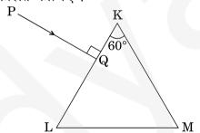
A triangular prism of refracting angle  $60^{\circ}$  is made of a transparent material of refractive index  $2/\sqrt{3}$ . A ray of light is incident normally on the face KL as shown in the figure. Trace the path of the ray as it passes through the prism and calculate the angle of emergence and angle of deviation.
