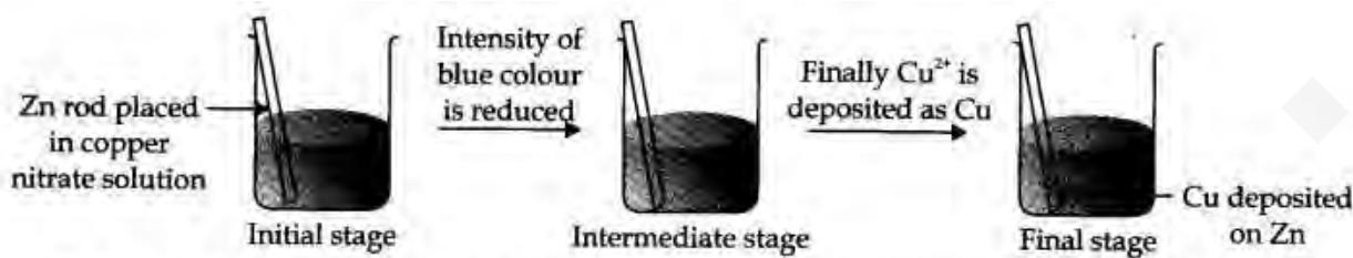
*Redox reaction between zinc and aqueous solution of copper nitrate occurring in a beaker.*
