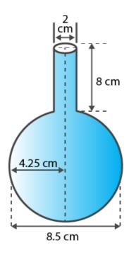
Now, the volume of this vessel = Volume of cylinder + Volume of a sphere
