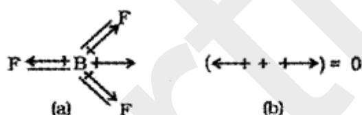
BF 3 molecule; representation of (a) bond dipoles and (b) total dipole moment
